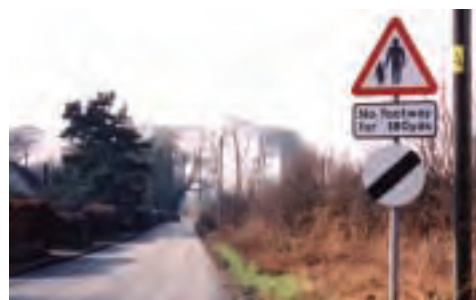
No footway and no speed limit is a potentially hazardous combination
