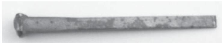
Figure 6: T-patent circa 1893 with chisel point
