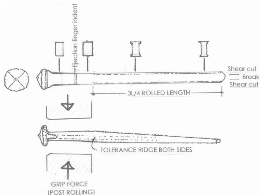
Figure 4: Ewbank nail features in the first two patents
